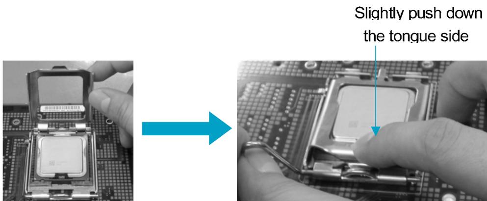
7. Lower the lever and lock it to the load plate, then the CPU is locked completely.
