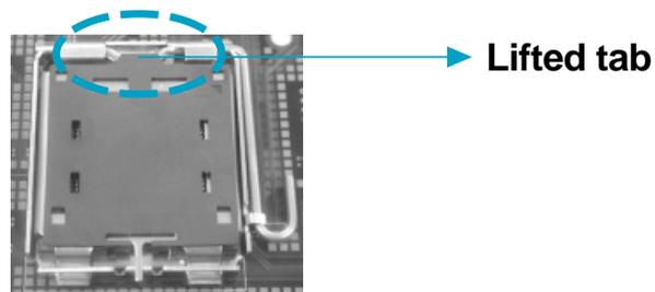
2. Lift the cap up and pick to upload the cap completely from the socket.
