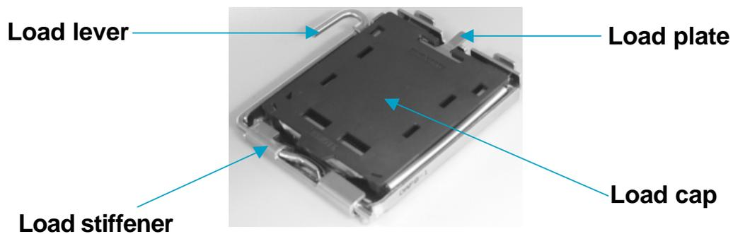
1. Use thumb & forefinger to hold the lifted tab of the cap.
